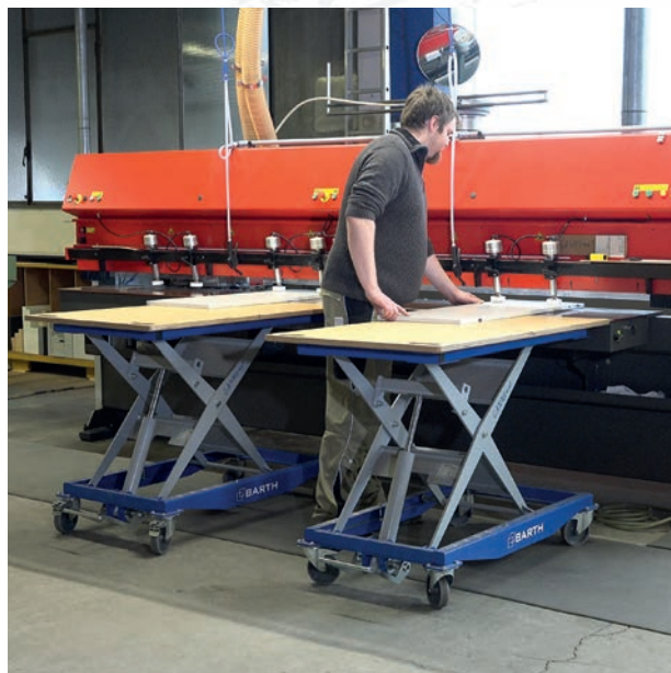
solid welded construction of the cylinder holder (maximum shear force 1.2 t)
