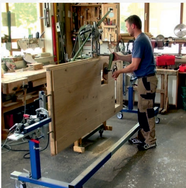
The wendoSYST can be equipped with a lifting table.
